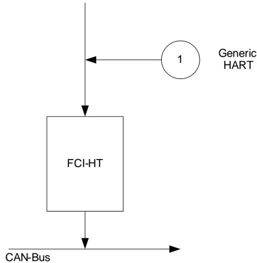
FIGURE 6-18 Analog mode system diagram
