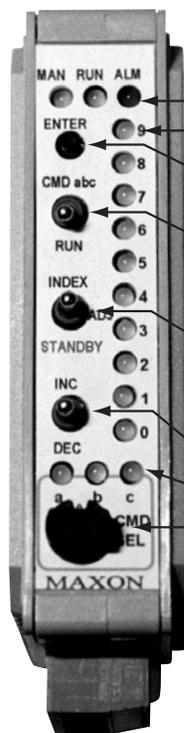
MAN Light - Unit in Manual Positioning Mode when lit.
